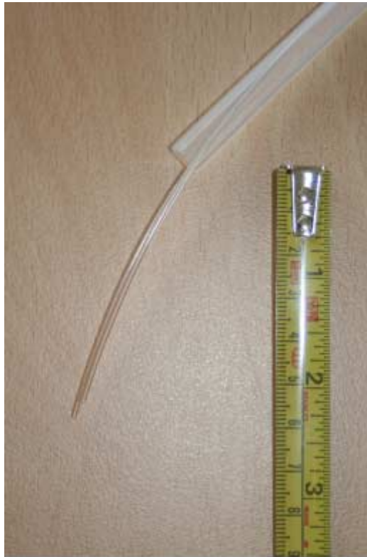
Figure 138 : The optical fibres will run inside protective teflon tubes in the detector
