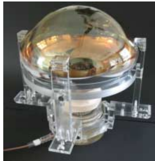
Figure 66 : Fig.-16: Drawing with present baseline dimensions and a picture of our prototype mechanical support assembled in one Hamamatsu 10" PMT.
