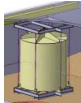
Figure 46 : Ties rod installation.
