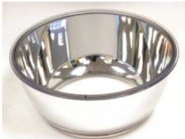
Figure 87 : Fig.-32: Prototype concentrator for approach using two nested acrylic forms.
